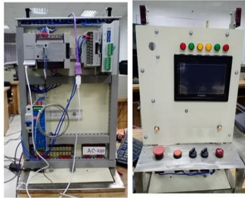
PLC, HMI testing module
